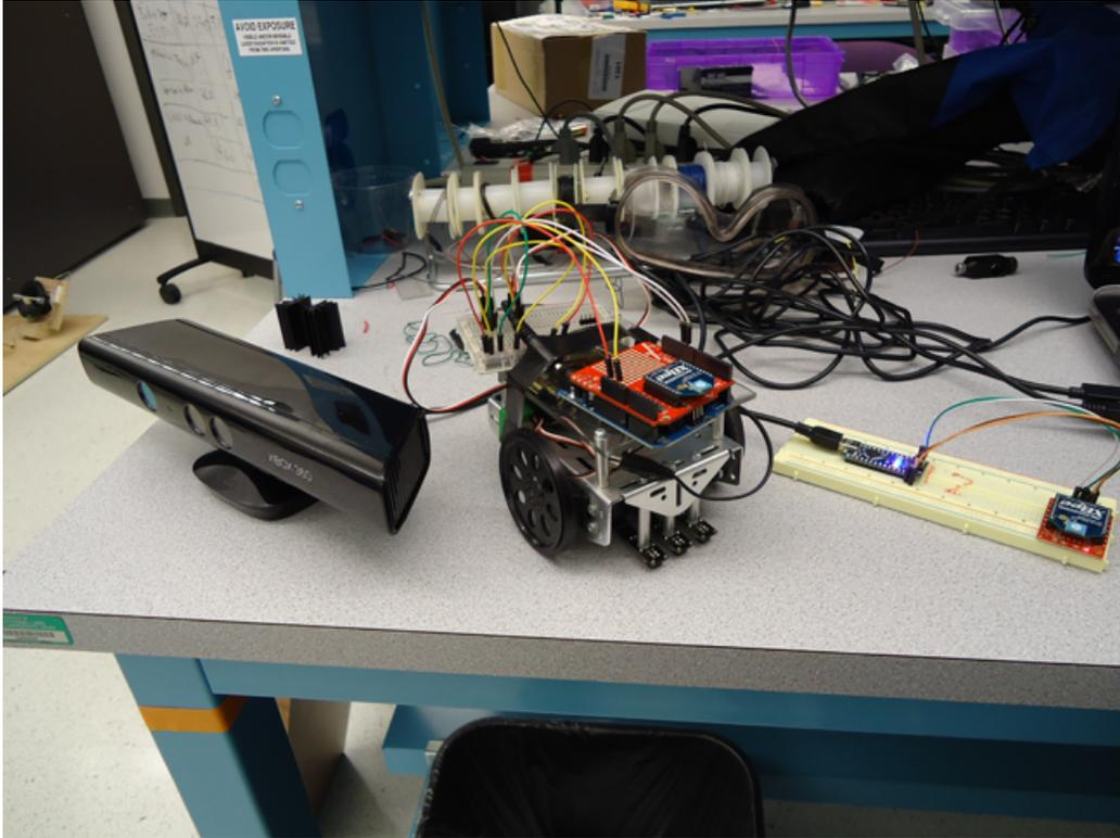
Figure 9: Kinect, Test Arduino MAAC application , and Transmitter System
